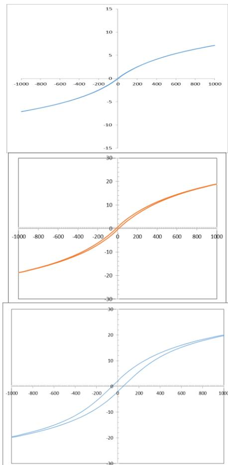
Fig.2: The hysteresis loops of MnFe<sub>2</sub>O<sub>4</sub> annealed at 0°C, 300°C and 500°C.
