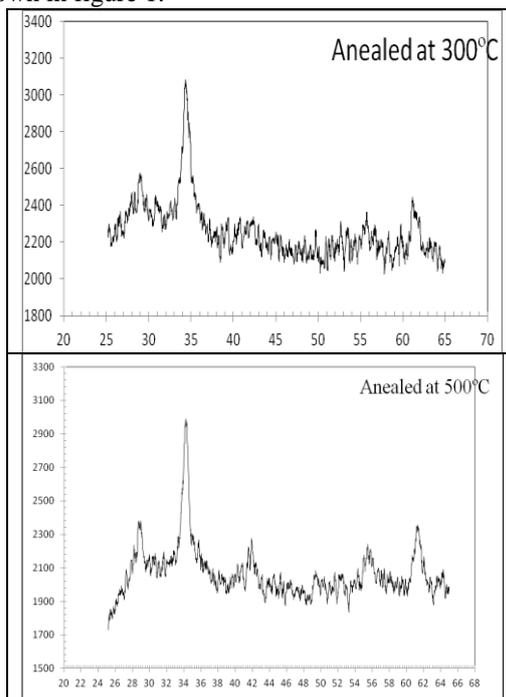
Figure1 shows that as the prepared sample consisted entirely of nano crystalline MnFe<sub>2</sub>O<sub>4</sub> particles.
