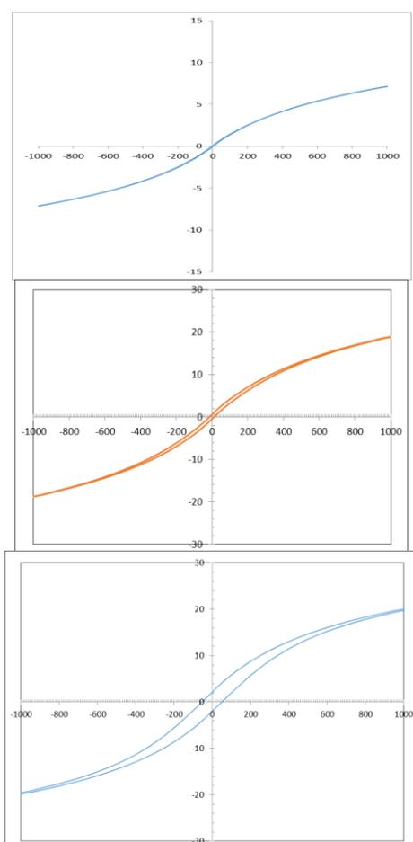
Fig.2: The hysteresis loops of  $MnFe_2O_4$  annealed at  $0^\circ C$ ,  $300^\circ C$  and  $500^\circ C$ .
